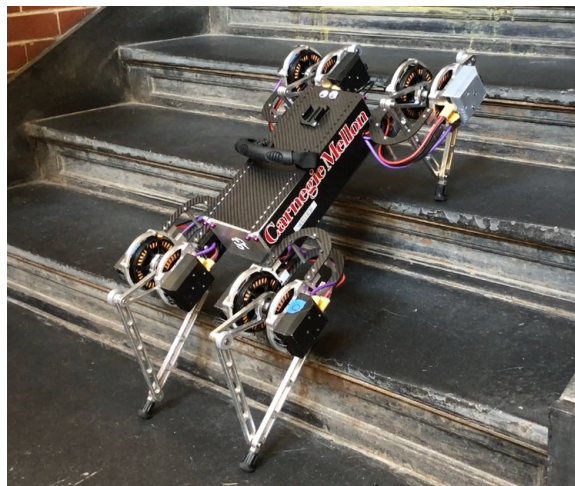
Fig. 1. Minitaur robot on the stairs used for testing.
